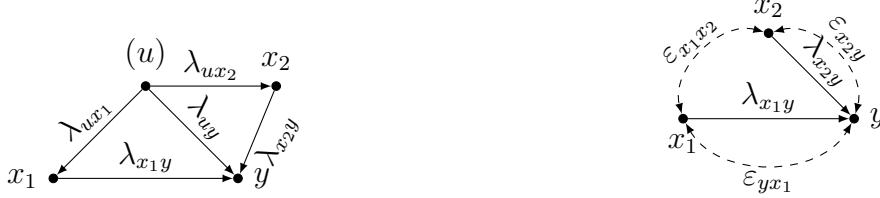
Figure 6.7: If two joint causes and one response are equiconfounded ( \lambda_{ux_1} = \lambda_{ux_2} = \lambda_{uy} ) this enables identification. Left: Latent variable DAG. Right: Latent projection.
