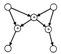
Figure 1. elimination of a crossover by use of "exclusive or" gates
